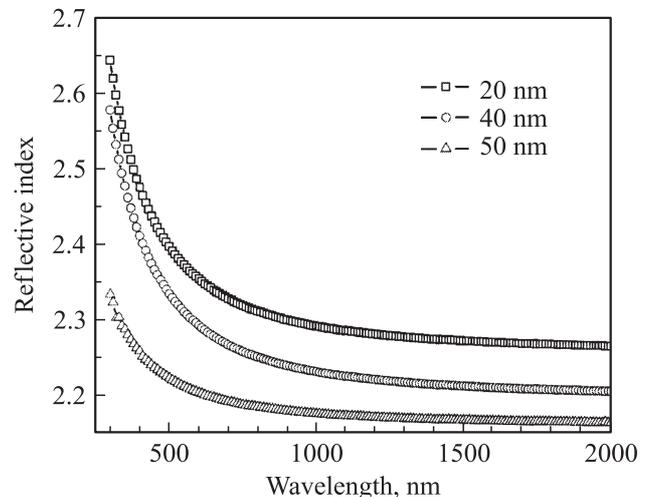
**Figure 6.** Refractive index of ZnS films deposited at various source-to-substrate distances.
