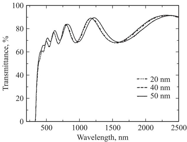
**Figure 4.** Transmission of ZnS films deposited at various source-to-substrate distances.
