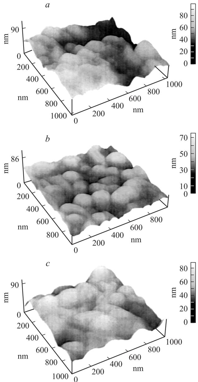
**Figure 3.** AFM images of ZnS films deposited at various source-to-substrate distances.
