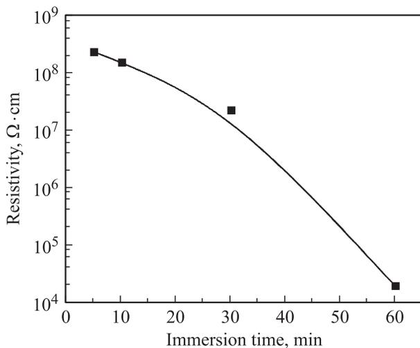
**Figure 7.** Resistivity versus immersion time of Ag doped ZnS films.
