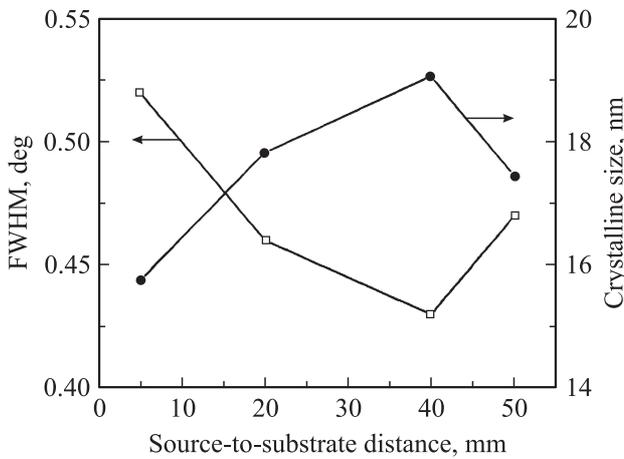
**Figure 2.** Variation of FWHM of (111) peak and crystallite size as a function of source-to-substrate distance.
