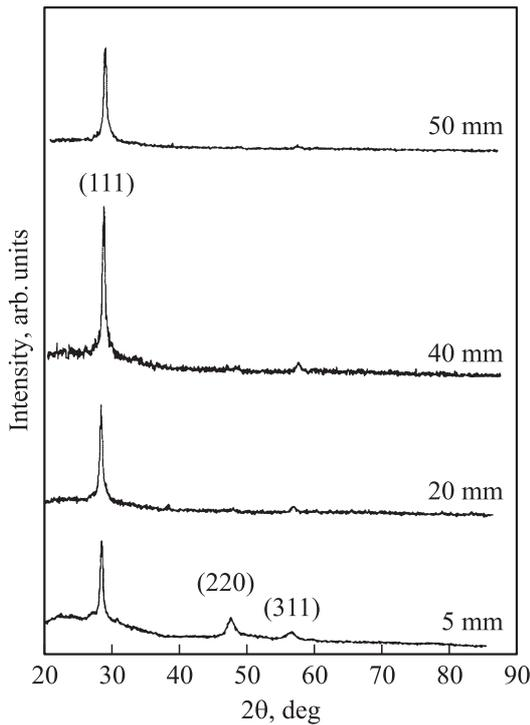
**Figure 1.** XDR pattern of ZnS films deposited at various source-to-substrate distances.
