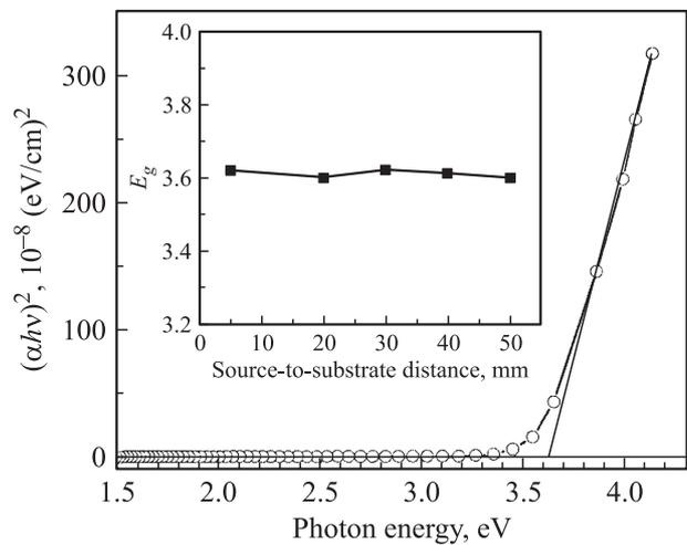
**Figure 5.** The  $(\alpha hv)^2$  versus photon energy for a ZnS film deposited at source-to-substrate distance of 40 mm. Inset shows energy bandgap of ZnS films as a function of source-to-substrate distance.
