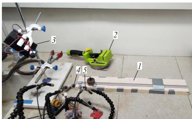
Figure 1. Photo of the experimental setup for initiating and recording the chemical transformation of the PS EC. Setup components: 1 — holder for samples CT-1 and CT-2, 2 — quick-release vice KITOKI BG-625702, 3 — laser diode GH04C05B9G in housing, 4 — copper induction coil used for thermal initiation of chemical transformation, 5 — photodetector FPU100-3. Near the left edge of the aluminum U-shaped profile, fixed on the stand, there is a punch, which can also be seen in Figure 4 and 5.
