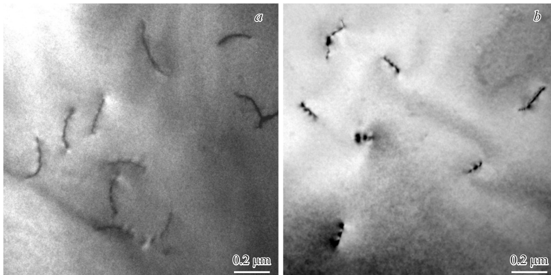
Figure 5. Light-field TEM-images of cross-sections in the planar geometry of a selectively grown GaAs layer in the central part of the window, obtained near the axis of zone [001]: a — sample 1, b — sample 2.
