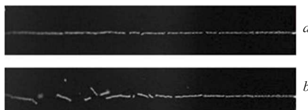
Figure 5. Collapse of the argon solid-phase jet at the reduced FC pressure: a — 6 \cdot 10^4 Pa, b — 4 \cdot 10^4 Pa. Shot by means of the high-rate video camera.
