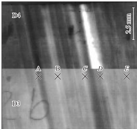
Figure 5. Intensity maps of D3 and D4 features in the photoluminescence spectrum. The letters A to E indicate the positions, where the spectra shown in Fig. 6 are taken.
