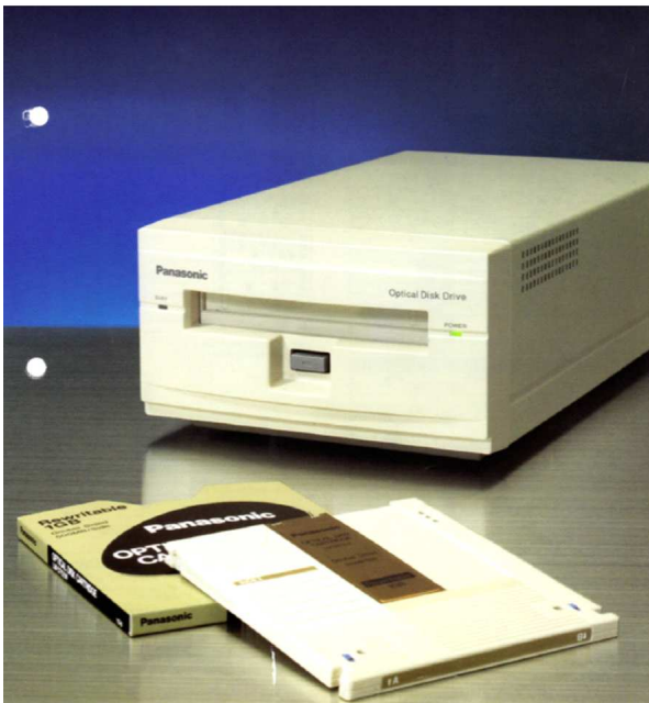
Figure 23. Photograph of the first optical disk based on phase-change materials and the corresponding receiving device (courtesy of N. Yamada).
