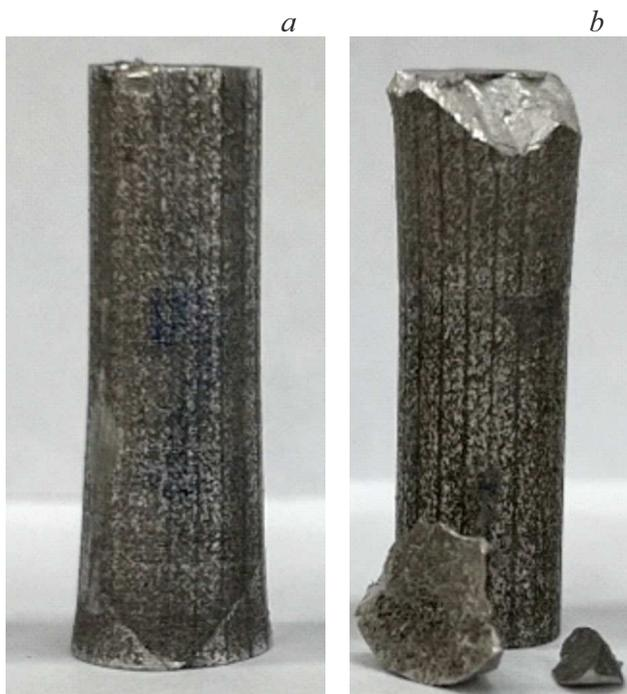
**Figure 2.** Fragments of the specimens after the impact tests: *a*) 219 m/s, *b*) 243 m/s).
