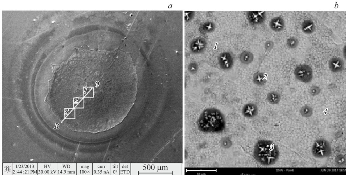
**Figure 1.** *a*) Area of laser impact with the M-pulse. Three zones 1–3 are shown: from the center of the focused laser beam (the zone 0) to the periphery (the zone R) of the laser beam with its impact on the surface. *b*) SEM-image of the zone 2 with arrangement of the dendrites on its surface (the digits denote points).
