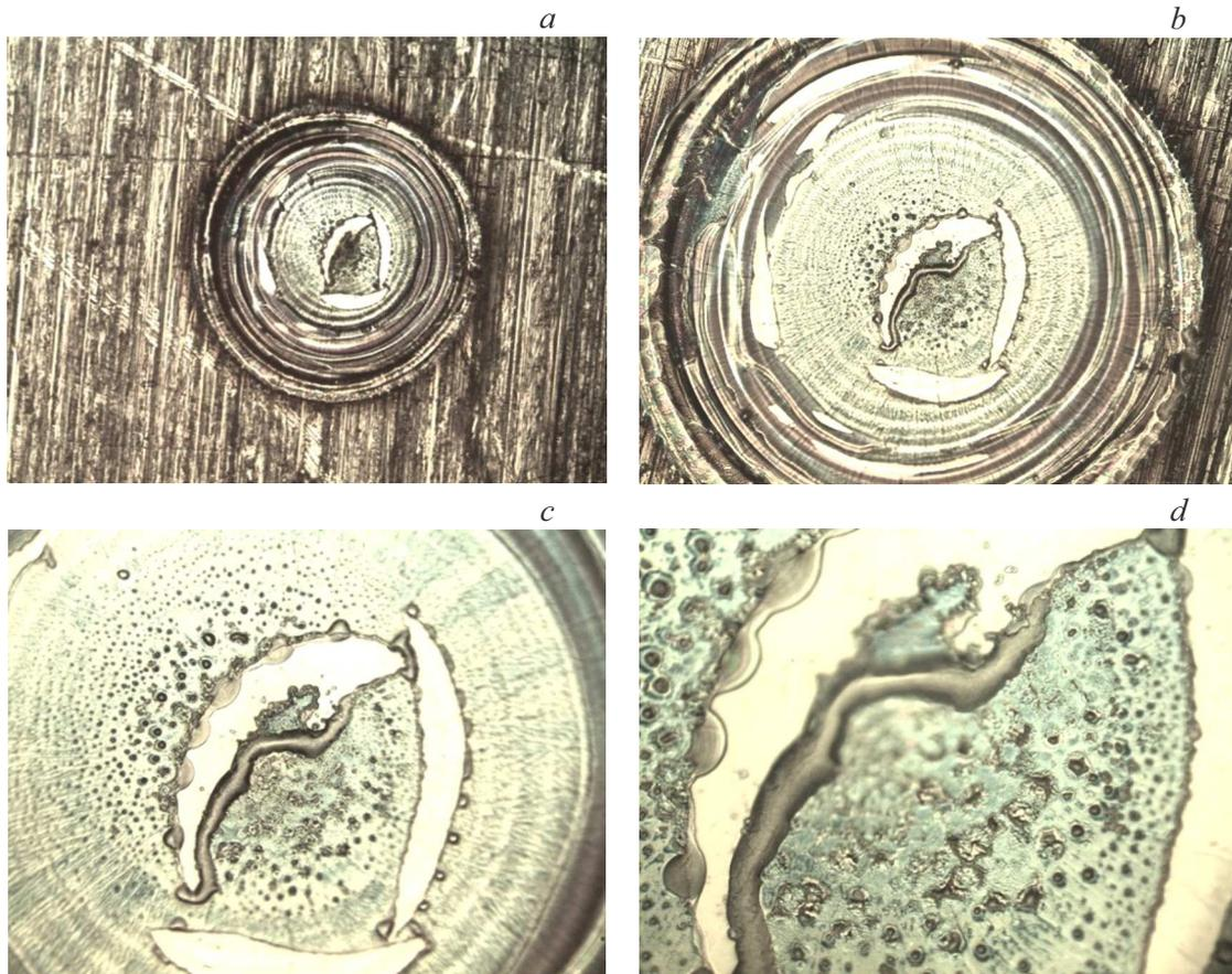
**Figure 5.** Optical microscopy of the laser-induced dendritic structure in the cavern on the surface of the stainless chromium-vanadium steel under different magnification: *a*)  $\times 125$ ; *b*)  $\times 250$ ; *c*)  $\times 500$ ; *d*)  $\times 1000$ .
