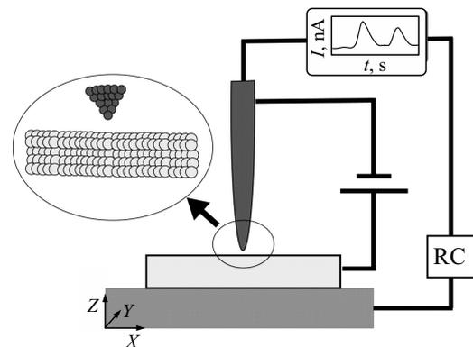
**Figure 7.** Schematic image of measurements of the I-V curves using the STM (see explanations in the text).
