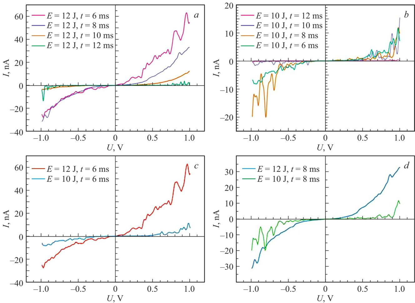
**Figure 8.** Graph of the dependence of the I-V curves of the dendritic microstructures formed at the constant energy of affecting laser radiation, which is 12 and 10 J for the different cases and at specified different durations of the laser pulses  $t$  (marked with a different color): *a*) when  $t = 6$  ms; *b*) when  $t = 8$  ms; *c*) when  $t = 10$  ms; *d*) when  $t = 12$  ms.
