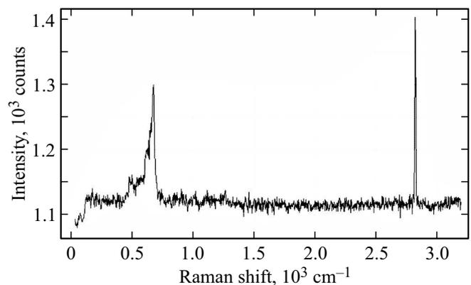
**Figure 4.** RS-spectrum obtained on one of the samples of the AISI 304 stainless steel with laser-synthesized dendrites on the surface of the solid sample.
