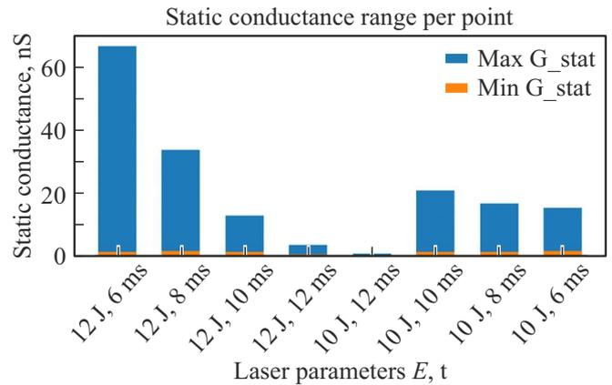
**Figure 9.** Diagram of variation of static conductance in a dependence on the laser radiation parameters specified on the abscissa axis (the energy  $E$  and the duration of the laser pulses  $t$ ).
