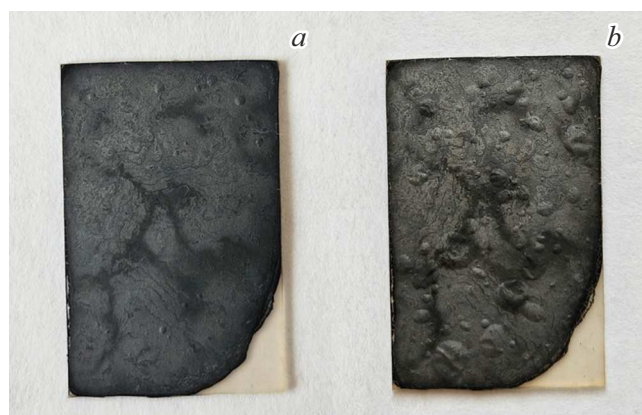
Figure 8. Photos of the Nafion-G-Pt/C composite film of the initial composition 14:56:30 before (a) and after (b) treatment with Fenton's reagent.
