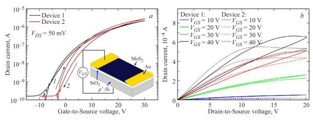
**Figure 1.** Transfer characteristics of the studied devices (a) and their output characteristics measured at different gate voltages (b). The inset shows a schematic drawing of the phototransistor structure of interest (photo-FET).
