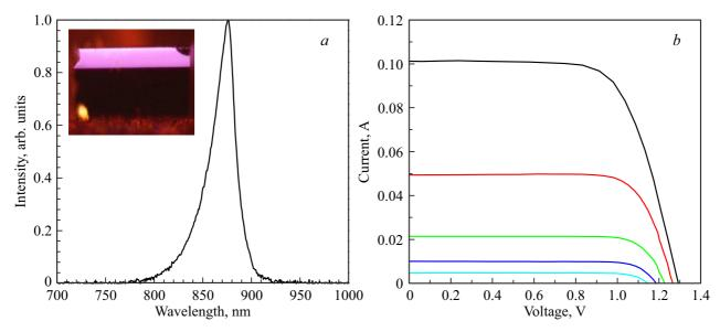
Figure 3. Micro-sized PVC characteristics: a — "edge" GaAs PVC electroluminescence spectrum and photo; b — IV-curves of "edge" GaAs PVC measured at various laser power densities.
