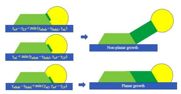
Figure 2. p-NW growth condition.
