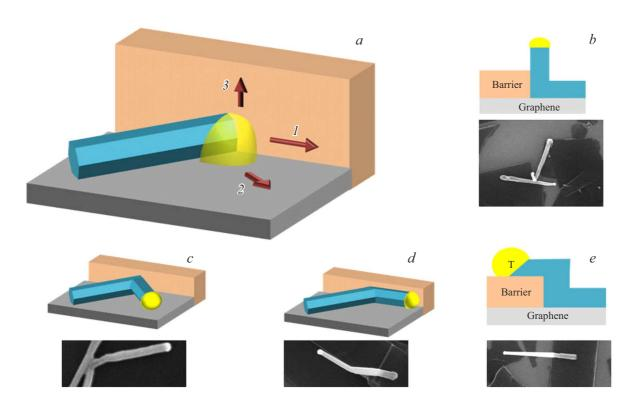
**Figure 3.** a — possible p-NW growth directions after coming in contact with the barrier; b — p-NW reflection from the barrier; c — continued NW growth along the barrier; d — inclined growth; e — continued growth through the barrier.
