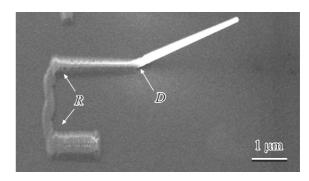
**Figure 1.** Change of the p-NW growth direction caused by a change of the doping level: rotation in plane — R, separation of p-NW — D.
