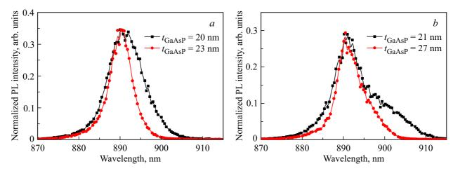
**Figure 2.** Normalized PL spectra for the InGaAs/AlGaAs heterostructures measured at low temperature (77 K) for samples with different CL thickness grown on wafers W2 (a) and W6 (b).
