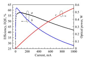
**Figure 3.** Dependences of the efficiency (a), external quantum efficiency (b) and optical power (c) of LED based on InGaAs MQW containing optimized GaAsP CL.
