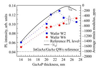
**Figure 1.** Dependence of the PL intensity maximum measured at room temperature on the GaAs<sub>0.92</sub>P<sub>0.08</sub> CL thickness for InGaAs/AlGaAs heterostructures grown on vicinal wafers W2 (squares) and W6 (circles). PL intensity level for the reference sample without CL is shown dashed, the solid line shows the calculated dependence of  $\varepsilon_a$  (Expression (1)).
