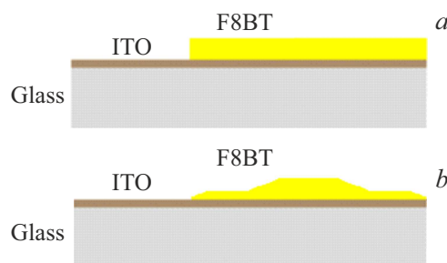
Figure 1. Sample structure. The ITO conductive substrate is coated with a F8BT polymer film. a — sample obtained by spin-coating (SC); b — sample obtained by drop casting (DC). The thickness of the films was 200–500 \mu\text{m} .
