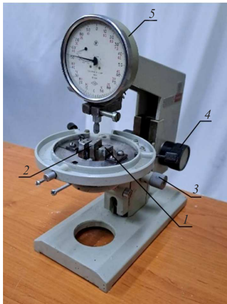
Figure 3. Homemade installation for measuring influence of strain on the thermoEMF of the thick-film thermoelectric sensor: 1 — the sample holder, 2 — the movable clamp, 3 — the handle for moving the clamp 2, 4 — the handle for moving the micrometer 5.
