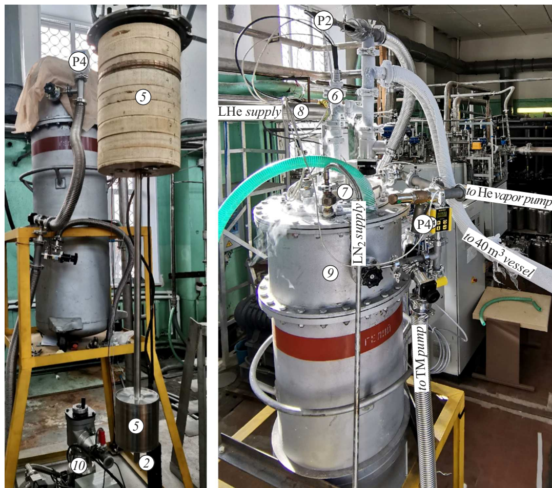
Figure 3. SOURCE vessel (in the left) and cryostat for obtaining IPH (in the right).
