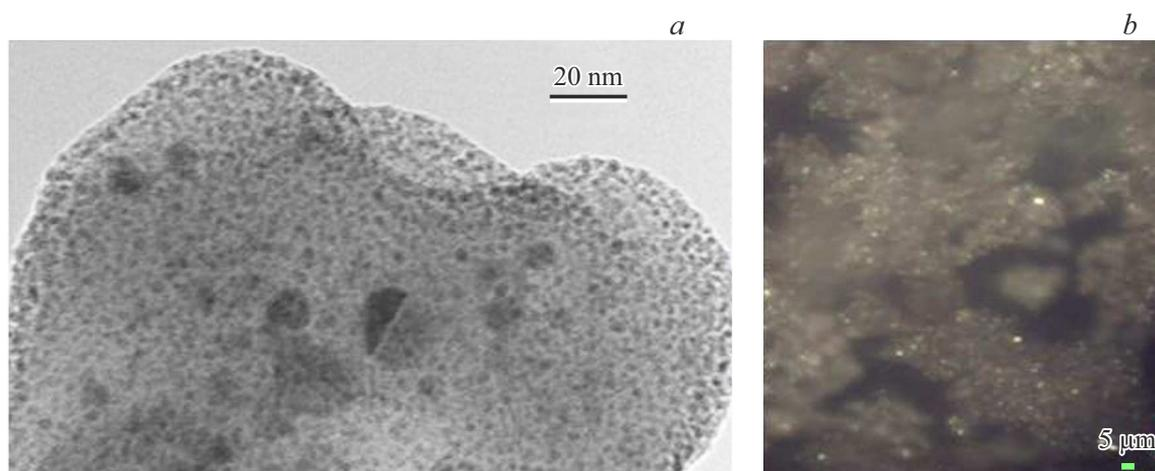
**Figure 1.** On the right — optical image of silver powder grains (in the solution). Scale bar at the bottom below —  $5\ \mu\text{m}$ . On the left — a structure of an individual grain in nanoscale.
