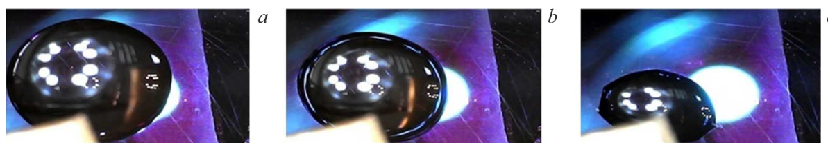
Figure 6. Drop evaporation on a surface characterized by \text{captionRms} = 23.1 \text{ nm} . Cases a–c correspond to 0, 50, 100 min after the start of observation of drop evaporation.
