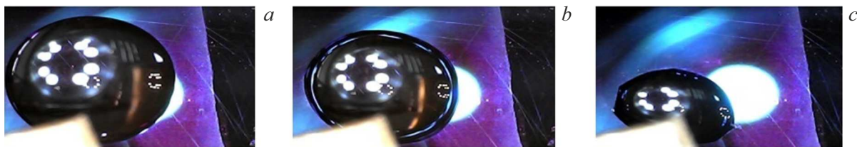
Figure 6. Drop evaporation on a surface characterized by R_{ms} = 23.1 nm. Cases a–c correspond to 0, 50, 100 min after the start of observation of drop evaporation.
