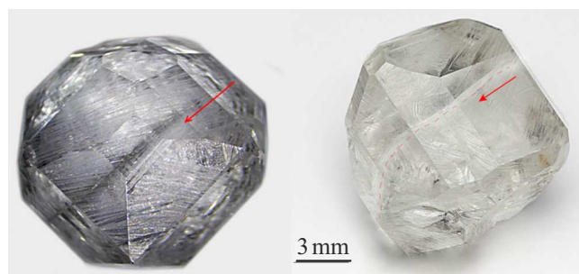
Figure 1. Crystals with horizontal (a) and vertical (b) cracks.
