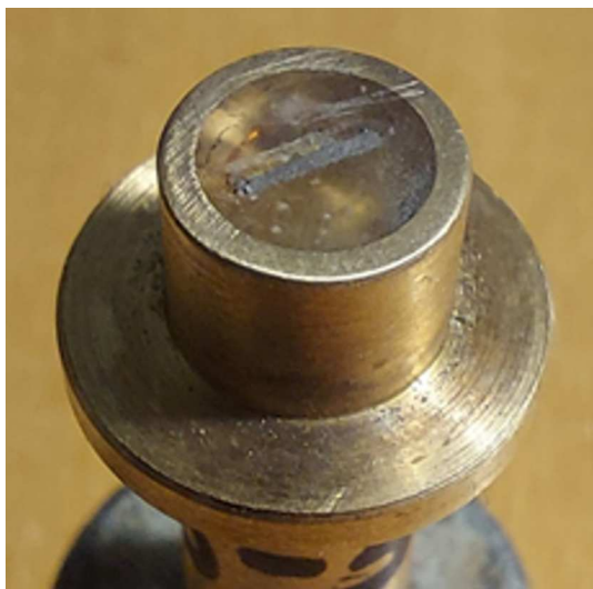
Figure 2. Insert with heat flux sensor on an anisotropic thermoelectric element made of single-crystal bismuth.
