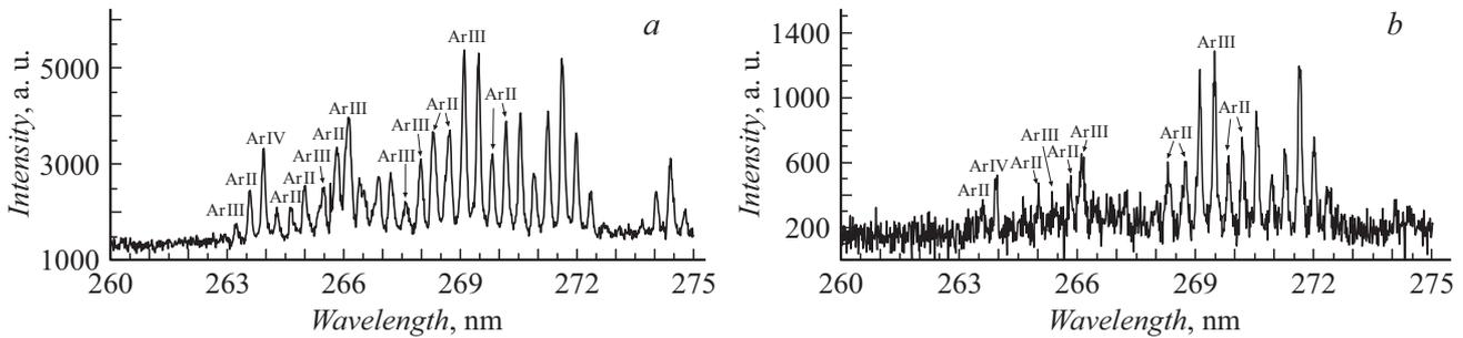
**Figure 2.** *a* — Spectrum of a discharge in an argon jet within the wavelength range of 260–275 nm (gas pressure in the discharge chamber, 0.35 bar; average FEL power, 200 W); *b* — spectrum of a discharge in an argon and nitrogen mixture within the 260–275 nm range (argon pressure in the injection line, 4 bar; background pressure of argon with added nitrogen, 0.3 bar; target–focus distance, 4 mm; average FEL radiation power, 200 W).
