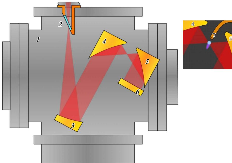
**Figure 1.** Discharge chamber (1) and diagram of FEL radiation input into it. 2 — Input window made of CVD diamond, 3 — 30° rotating mirror, 4 and 5 — 90° focusing mirrors, 6 — planar mirror, and 7 — gas injection tube.
