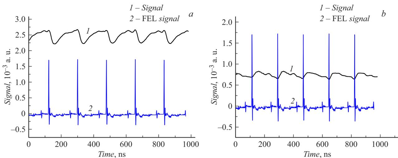
**Figure 3.** Time dependence of the photodiode signal (1) and the FEL radiation signal (2). *a* — Discharge in an argon jet; *b* — discharge in an argon jet with nitrogen added to the argon buffer volume.
