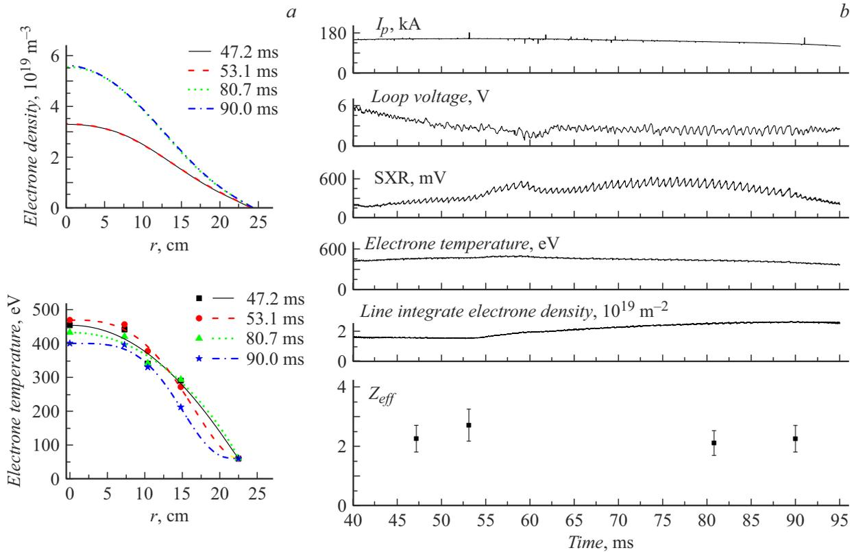
**Figure 2.** *a* — Radial profiles of electron density  $n(r)$  (top) and temperature  $T(r)$  (bottom) for different time intervals. *b* — Plasma parameters (top to bottom): current, loop voltage, X-ray radiation, maximum electron temperature at the center, chord-averaged electron density, and effective charge. Discharge No. 24032706. A color version of the figure is provided in the online version of the paper.
