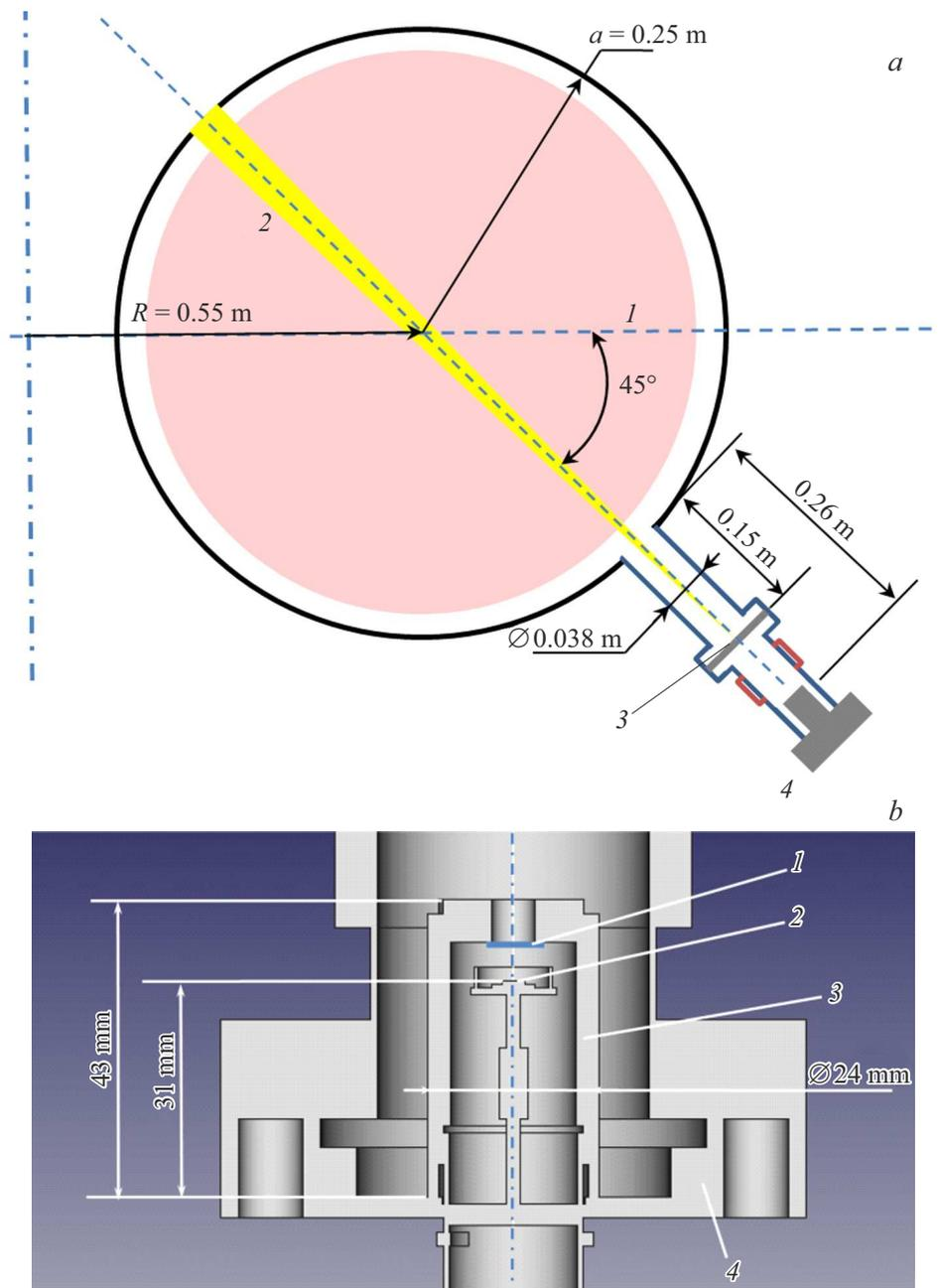
**Figure 1.** *a* — Diagram of detector installation at a TUMAN-3M tokamak, poloidal section. *1* — Plasma column, *2* — detector field of view, *3* — diaphragm, and *4* — detector. *b* — Internal structure of the detector. *1* — Beryllium foil, *2* — sensitive element, *3* — cap, and *4* — flange.
