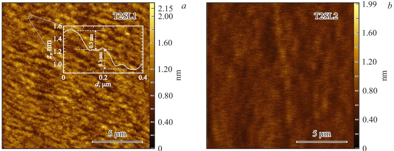
**Figure 1.** AFM images of the T2SL1 (a) and T2SL2 (b) surfaces. Steps approximately 100 nm wide and 0.3 nm high are visible, which matches with the monolayer height of the terrace.
