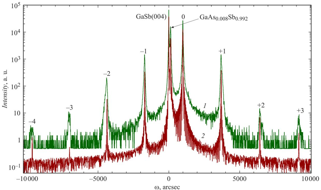
**Figure 2.** Experimental (1) and calculated (2) diffraction reflection curves obtained in the geometry of symmetric reflection (004) for the T2SL2 sample.
