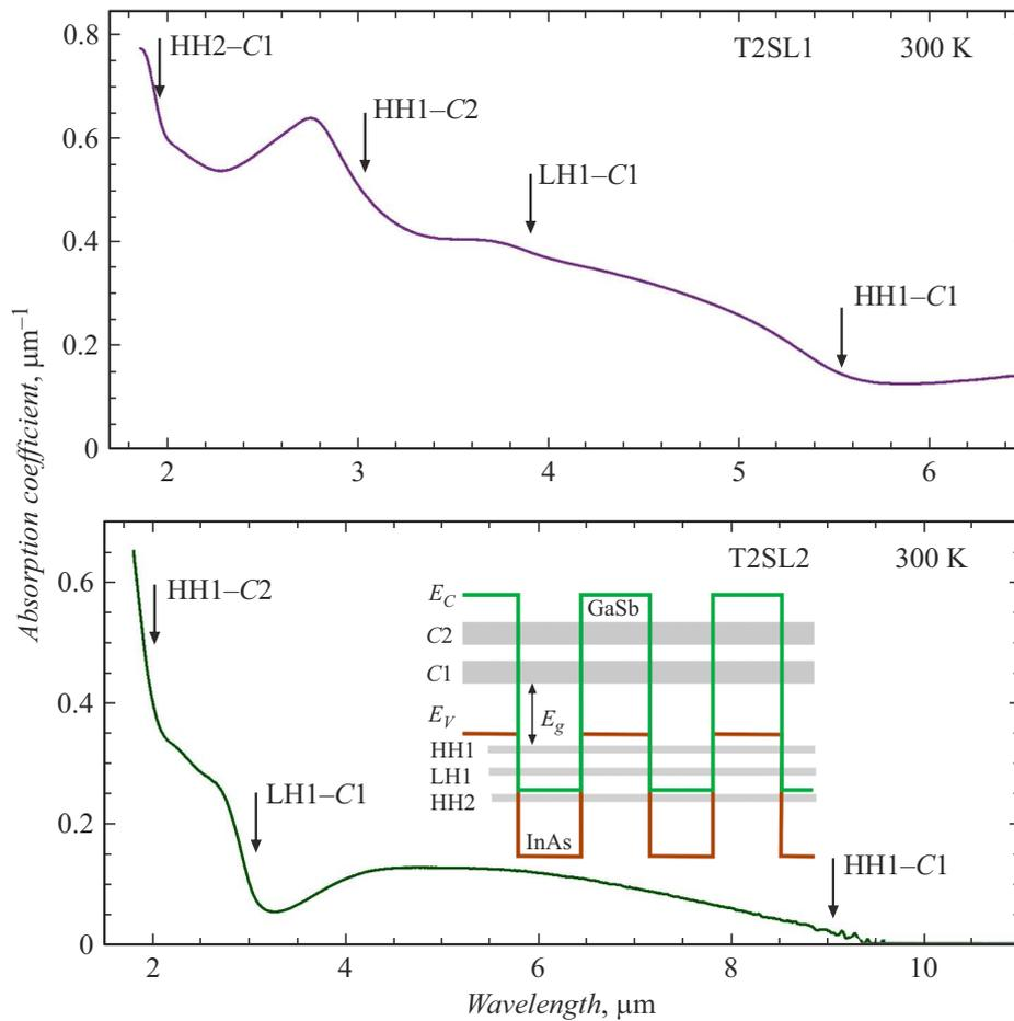
**Figure 3.** Superlattice absorption spectra. The inset schematically represents the edges of the InAs and GaSb conduction and valence bands, as well as minibands of electrons (C1 and C2), heavy holes (HH1 and HH2) and light holes (LH1) emerging in the superlattice. Arrows indicate the transition points as per [13].
