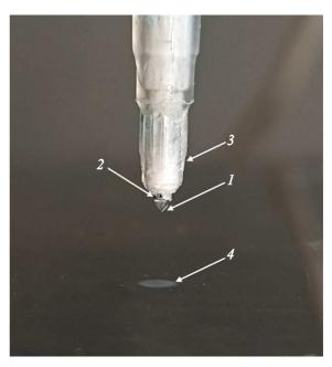
**Figure 2.** Spraying of a  $\text{TiO}_2$  nanopowder suspension onto a polished LDI target. I — Meniscus of the sprayed suspension in the droplet-free mode, 2 — end face of the metal capillary, 3 — outer coaxial dielectric capillary, and 4 — dry mechanically stable  $\text{TiO}_2$  spot.
