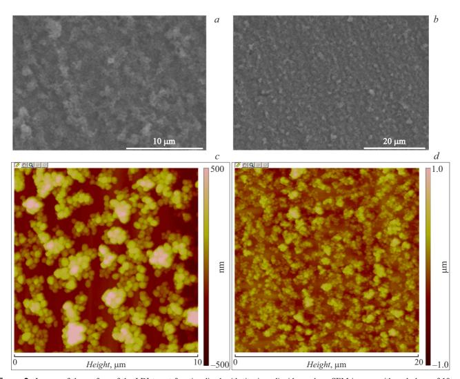
**Figure 3.** Images of the surface of the LDI target functionalized with titanium dioxide. a, b — SEM images with scale bars of 10 and  $20 \,\mu\text{m}$ ; c, d — AFM images with frame sizes of  $10 \times 10$  and  $20 \times 20 \,\mu\text{m}$ .
