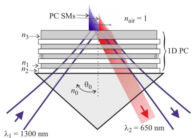
**Figure 1.** Experimental setup. PC SMs are PC surface modes, 1D PC is the one-dimensional PC (not to scale).
