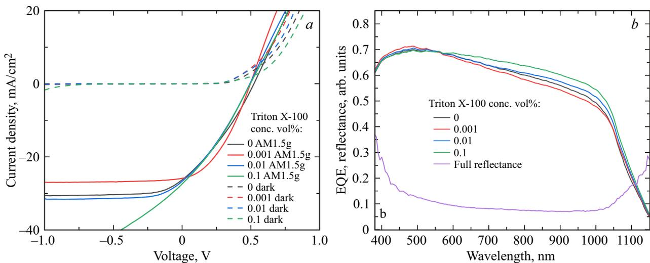
**Figure 3.** Current-voltage curves (*a*) and spectra of EQE and full reflection (*b*) of photoconverter structures based on heterojunction PEDOT:PSS/*n*-Si, obtained on surface of array of silicon fibers.
