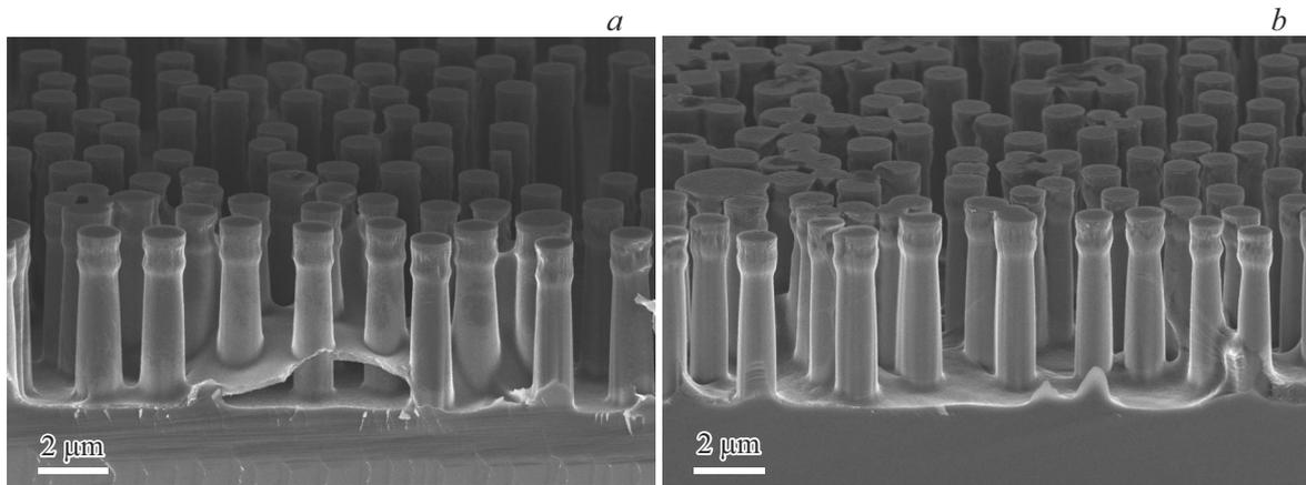
**Figure 2.** SEM-image of vertically oriented Si structures coated with layer PEDOT:PSS without addition of Triton X-100 (*a*) and with addition of 0.1 vol% of Triton X-100 (*b*).
