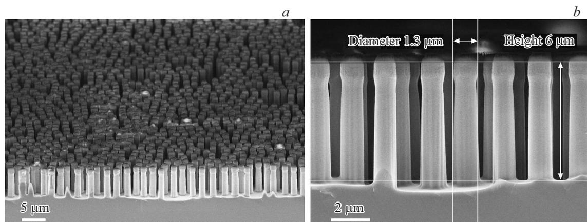
**Figure 1.** SEM-images of surface of vertically oriented Si structures (a) and individual fibers (b) on substrate of crystalline silicon obtained by method of microsphere lithography and cryogenic plasma-enhanced chemical etching.
