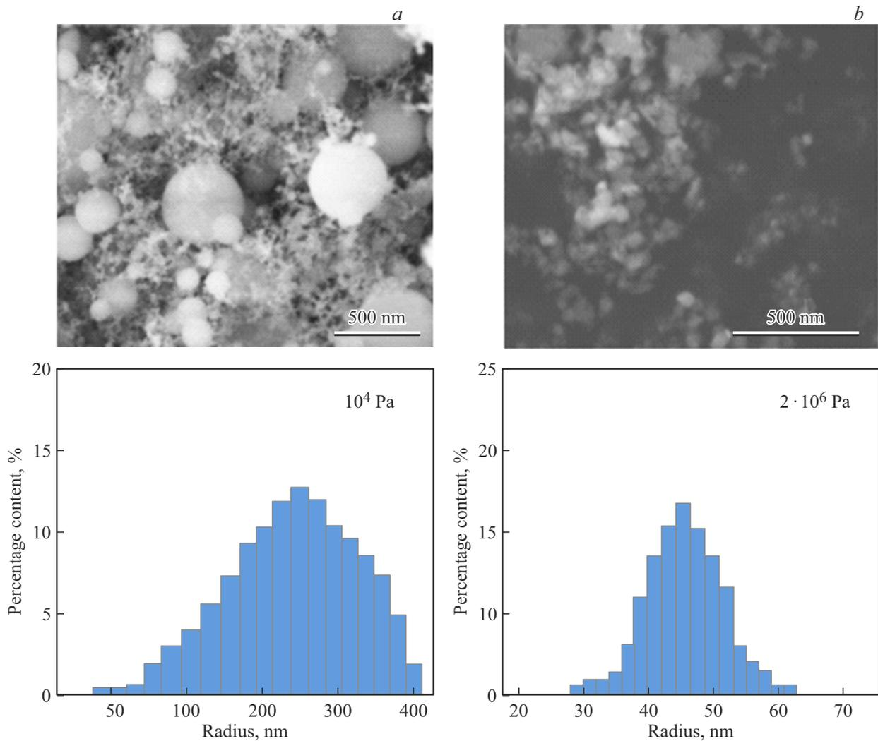
**Figure 1.** Histograms of distribution by size of ZnS particles and corresponding SEM images. *a* — particles synthesized at argon pressure of  $10^4$  Pa, *b* — at argon pressure of  $2 \cdot 10^6$  Pa.
