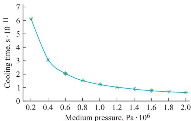
**Figure 2.** Dependences of mean time of particle cooling to 500 K on buffer gas pressure.
