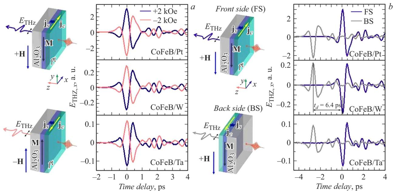
**Figure 2.** Analysis of the THz generation mechanisms in bilayer CoFeB/(Pt,W,Ta) structures. *a* — investigation of the effect of the external magnetic field  $\mathbf{H}$  polarity on the THz signal temporal dynamics; *b* — investigation of the effect of direction of the structure irradiation with a laser pulse on the generated THz signal phase under the applied magnetic field with the same polarity.
