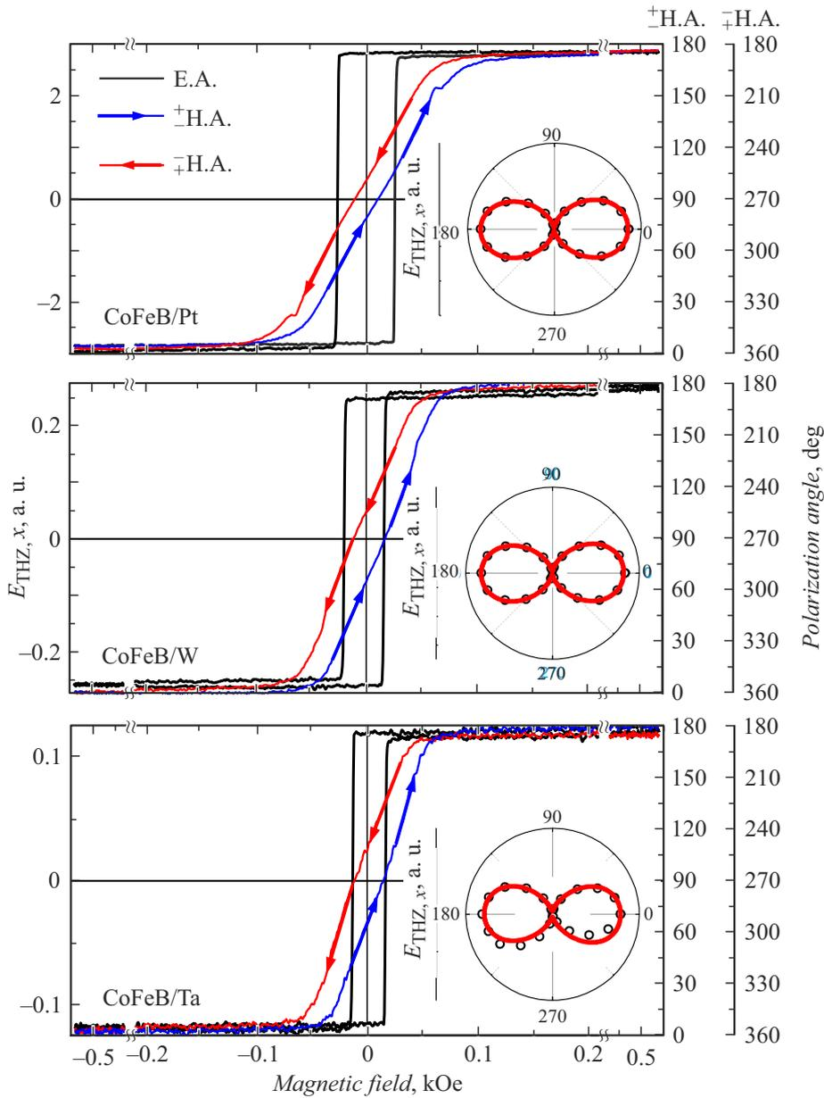
**Figure 3.** Magnetic hysteresis loops of the THz signal in the CoFeB/(Pt,W,Ta) structures. The insets present polarization-angle dependences of the THz amplitude  $E_x$ , which have been measured in the magnetic field of +2 kOe by rotating the THz polarizer.
