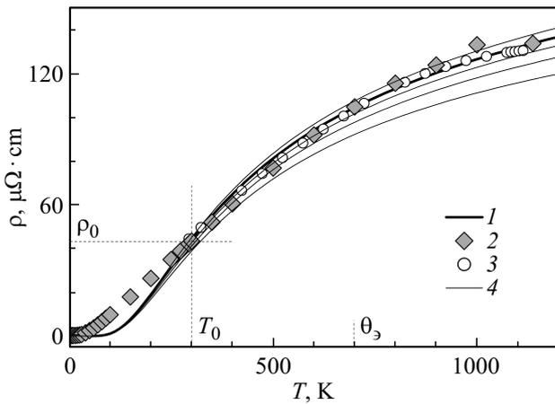
**Figure 5.** High-temperature isobars of electrical resistivity  $\alpha$ -Zr. 1 — model atmospheric isobar  $\rho = \rho(V, T)$ . 2 — recommended experimental values for atmospheric isobar from [2]. 3 — recommended experimental values from [3]. 4 — model isobars of electrical resistivity of zirconium under pressures (from top down) –1.0, 1.0, 2.5 and 5.0 GPa.
