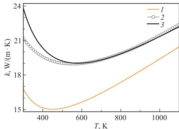
**Figure 6.** Thermal conductivity  $k$  of zirconium  $\alpha$ -Zr vs. temperature  $T$  along atmospheric isobar. 1 — electronic component  $k_e$ . 2 — generalization of experimental isobars of thermal conductivity at atmospheric pressure (5) from [4]. 3 — sum of electronic and lattice components  $k = k(V, T) = k_e + k_l$  (6).
