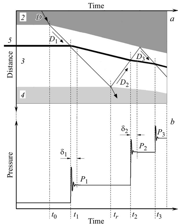
**Figure 2.** Operation of generator of step-like cyclic shock loading. (*a*) Kinematics of shock waves in coordinates Distance–Time, symbols *2, 3, 4, 5* mean same as in Figure 1. (*b*) Profile (dependence on time) of pressure in sample under study. Symbols in Figure 2, *b* are explained in text.
