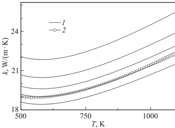
**Figure 7.** Temperature-baric dependence of thermal conductivity  $\alpha$ -Zr at high temperatures and pressures. 1 — model isobars of thermal conductivity at pressure (from bottom to top)  $-1.0, 0.0, 1.0, 2.5, 5.0$  GPa. 2 — fragment of graph (5) generalizing experimental isobars of thermal conductivity at atmospheric pressure from [4].
