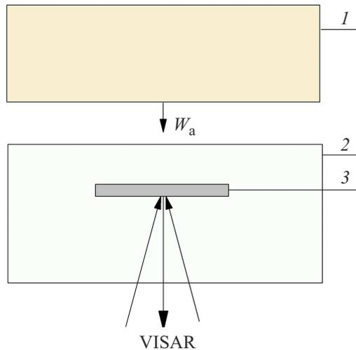
**Figure 8.** Scheme of experiment on recording the profile  $u(t)$  (dependence on time  $t$ ) of mass speed of frontal surface of sample. 1 — copper impactor with diameter 48.0 mm and thickness 2.5 mm flying at speed  $W_a = 347 \text{ m/s}$ , 2 — plexiglass block with diameter 50 mm and thickness  $\sim 10 \text{ mm}$ , 3 — zirconium sample  $\sim 20 \text{ mm}$  in diameter and  $h_0 = 0.20 \text{ mm}$  thick, rare surface of sample is at distance 2.0 mm from rare surface of block 2.
