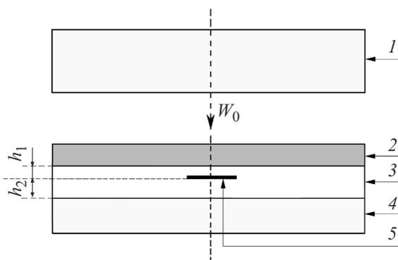
**Figure 1.** Generator of step-like shock-wave loading. *1* — aluminium impactor, *2* — steel or tungsten plate, *3* — teflon, *4* — steel or tungsten plate, *5* — tape sample  $h_0 = 0.045(5)$  mm thick and  $a_0 = 1.90(5)$  mm wide.
