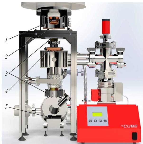
Figure 1. Setup for irradiating materials with an electron beam (the central part is a cutaway view): 1 — LaB6 electron thermal emitter; 2 — accelerating anode (8.5 kV); 3 — focusing coils; 4 — longitudinal and transverse bias coils; and 5 — material sample.
