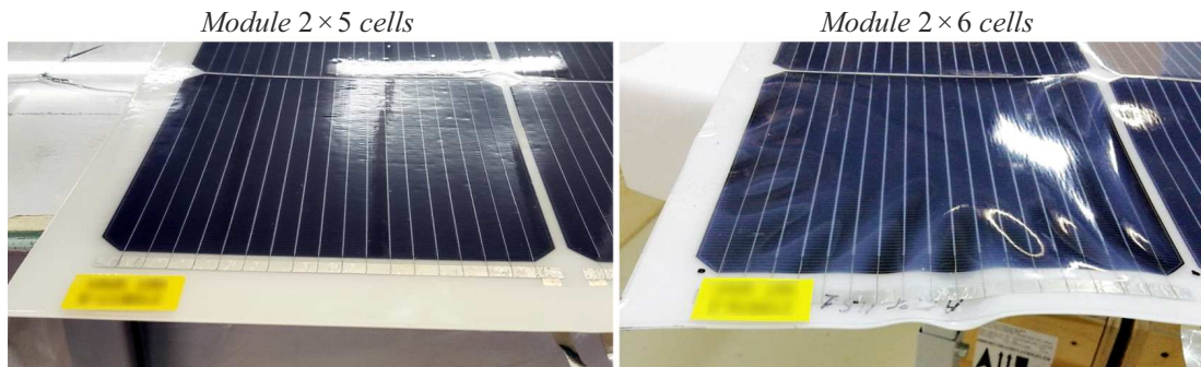
Figure 6. Deformation of a semi-flexible PVM containing 2 \times 6 PVCs and lack of deformation of a PVM containing 2 \times 5 PVCs after hot spot testing.
