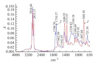
**Figure 6.** IR spectra of samples of natural rubber SVR-10 (*1* (red curve) — original rubber, *2* (blue curve) — dried rubber extract).
