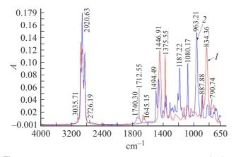
**Figure 5.** IR spectra of samples of rubber SKI-5 PM (1 (red curve) — original rubber, 2 (blue curve) — dried rubber extract).
