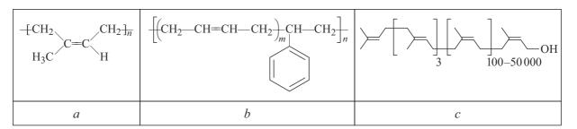
**Figure 1.** Structural formulas of the objects of research: a — structural formula of SKI-5 PM rubber (*cis*-1,4-isoprene); b — structural formula of SKMS-30 ARKM-27 rubber; c — the structural formula of NR.
