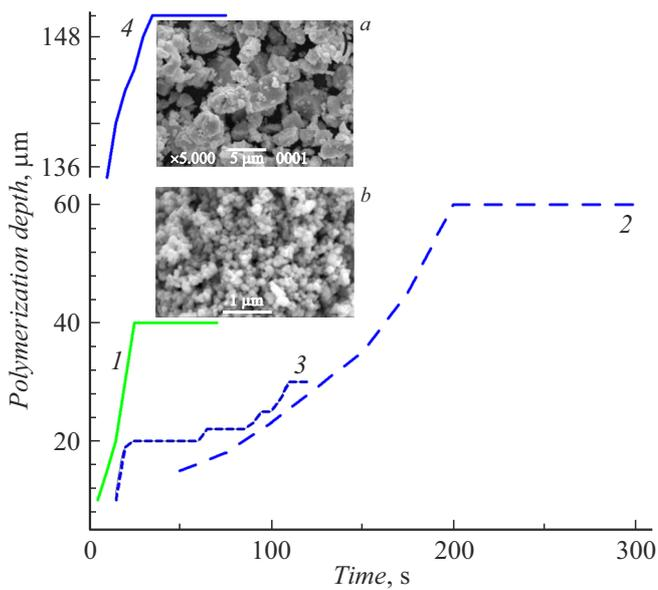
**Figure 1.** Photopolymerization depth of 3D samples of pastes with BT and PZT as a function of exposure time. 1 — 37 vol.% BT, the mean ceramic particle size is  $0.25\ \mu\text{m}$ ; 2 — 50 vol.% PZT,  $2\ \mu\text{m}$ ; 3 — 37 vol.% PZT,  $3.5\ \mu\text{m}$ ; 4 — 37 vol.% PZT,  $5\ \mu\text{m}$ . SEM images of the initial piezoceramic powders are shown in the insets: PZT (a) and BT (b).
