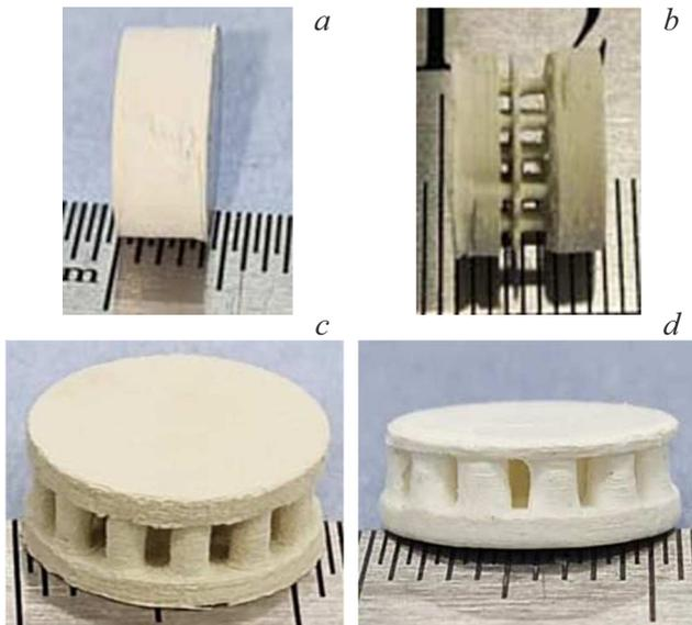
**Figure 2.** External view of 3D-printed HLSs with different types of topological connectivity. *a* — Solid PZT (0–3), *b* — PZT (3–3), *c* — PZT (1–3), and *d* — BT (1–3). The ruler scale interval is 1 mm.
