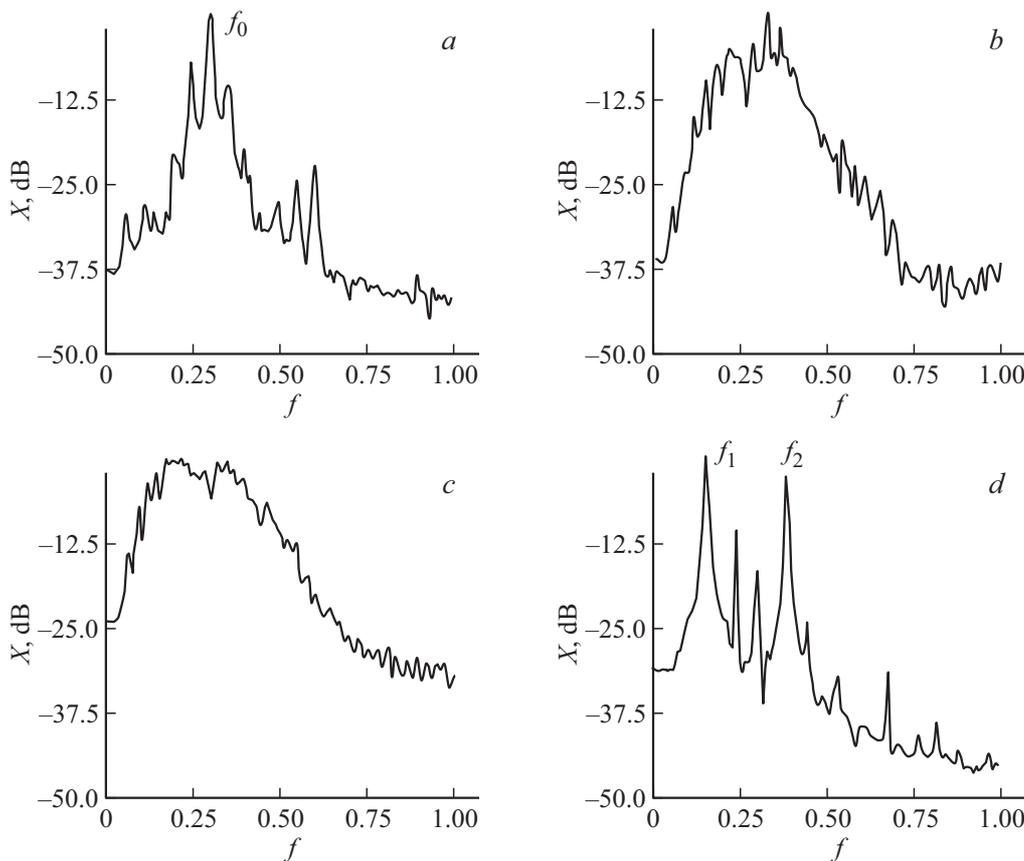
**Figure 1.** Dynamics of the oscillatory process of a system of two coupled GDIs with variation of the coupling coefficient between partial oscillators:  $k = 0.1$  (a),  $0.42$  (b),  $0.53$  (c) and  $0.61$  (d).
