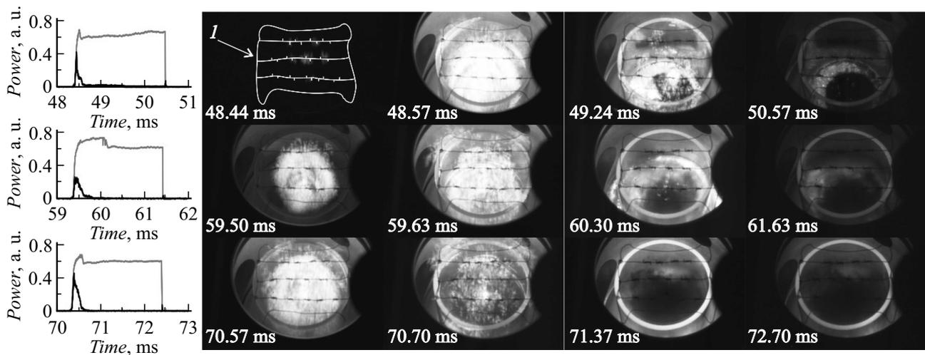
**Figure 1.** Frames (the exposure time is  $130\ \mu\text{s}$ ) illustrating the evolution of a microwave discharge. The top, middle, and bottom rows correspond to the first, second, and third pulses in a sequence. *1* — Outline of the initiator of the microwave subthreshold discharge in the form of a nickel wire. The insets present the temporal variation of gyrotron radiation power (gray curve) and power transmitted through the powder sample and the plasma-dust cloud (black curve).
