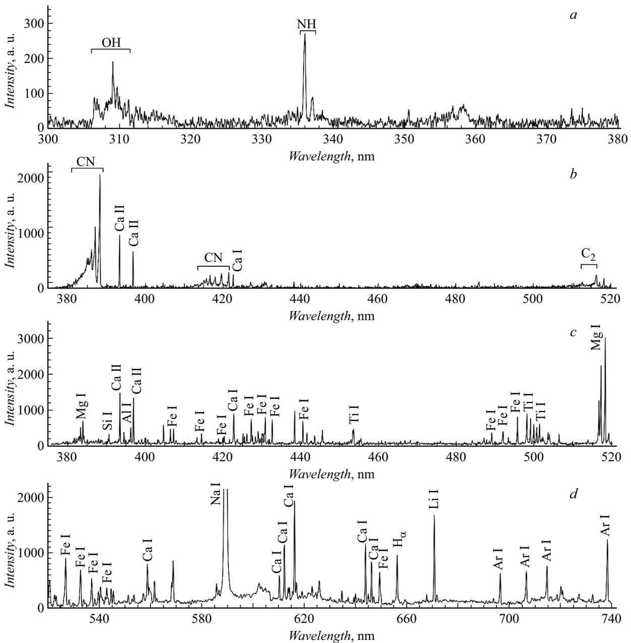
**Figure 3.** Fragments of discharge emission spectra. *a, b* — First pulse; *c, d* — third pulse.
