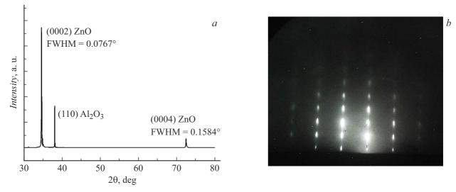
**Figure 1.** a - XRD pattern of an epitaxial ZnO film; b - reflection electron diffraction pattern for an epitaxial ZnO film (the electron energy is 75 keV).
