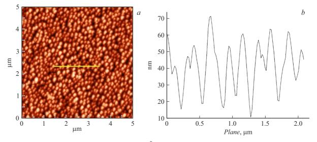
**Figure 3.** a — surface topography of the (0001)ZnO  $\| (11\overline{2}0)Al_2O_3$  film; b — profile of the section along the indicated line.
