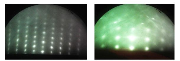
**Figure 2.** Reflection electron diffraction patterns recorded at two different azimuth angles for an epitaxial ZnO film obtained at a temperature of 35°C,  $j = 33 \text{ mA/cm}^2$ , t = 30 min,  $h = 5 \mu \text{m}$ , and v = 2.8 nm/s.
