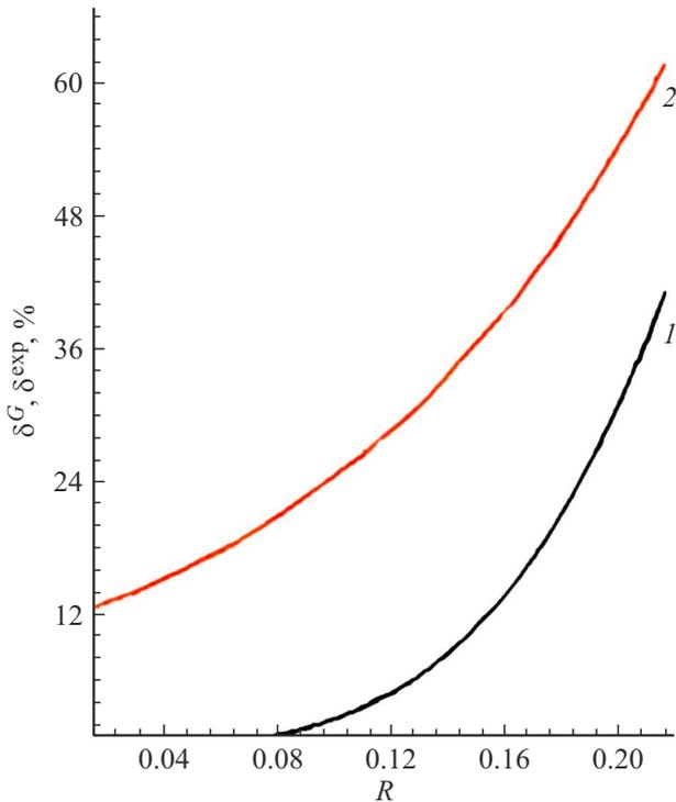
**Figure 2.** Dependence of the second moment measurement error on  $R$  at  $T = 0.01$  m for (1) the Gaussian  $\delta^G(R)$  and (2) exponential  $\delta^{\text{exp}}(R)$  spatial intensity distributions in the emitter plane.
