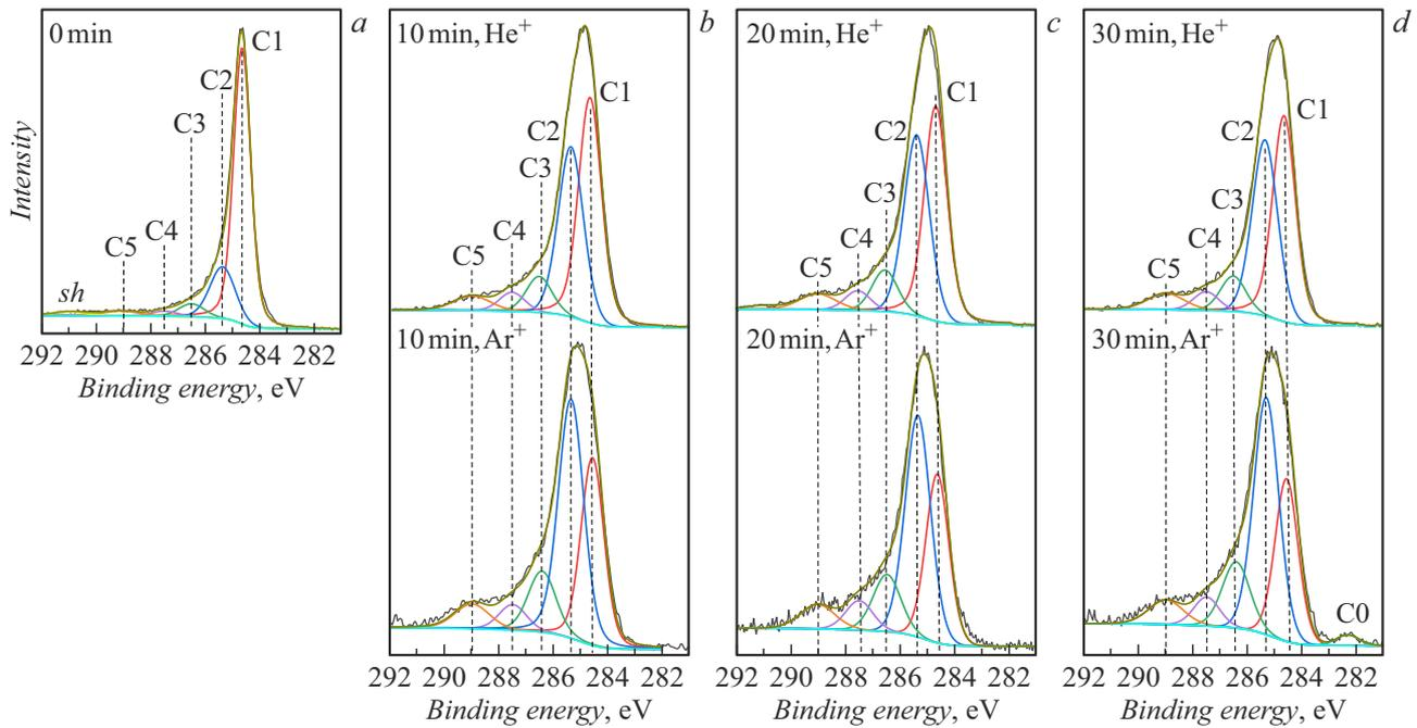
**Figure 4.** C 1s PE spectra of the surface layer of „MWCNT/Ti“ samples: before irradiation (a) and after 10 (b), 20 (c) and 30 min (d) irradiation with helium and argon ions.
