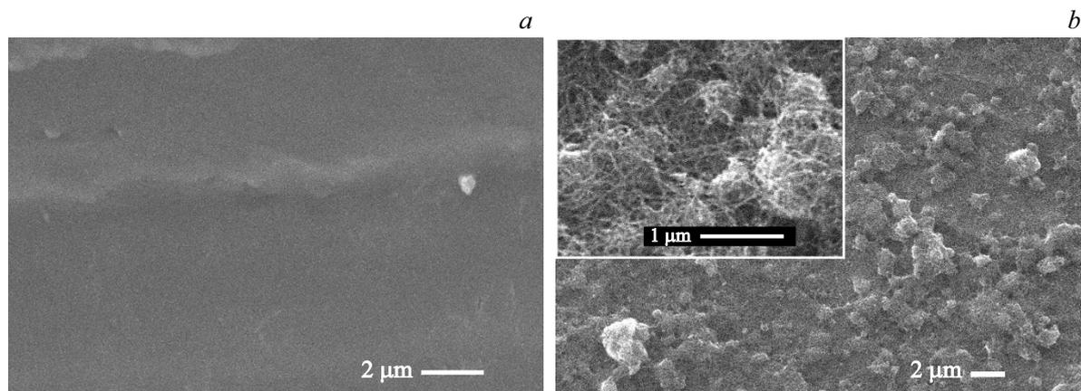
**Figure 1.** SEM images of the Ti substrate surface (a) and the surface layer of „MWCNT/Ti“ system (b) before irradiation.
