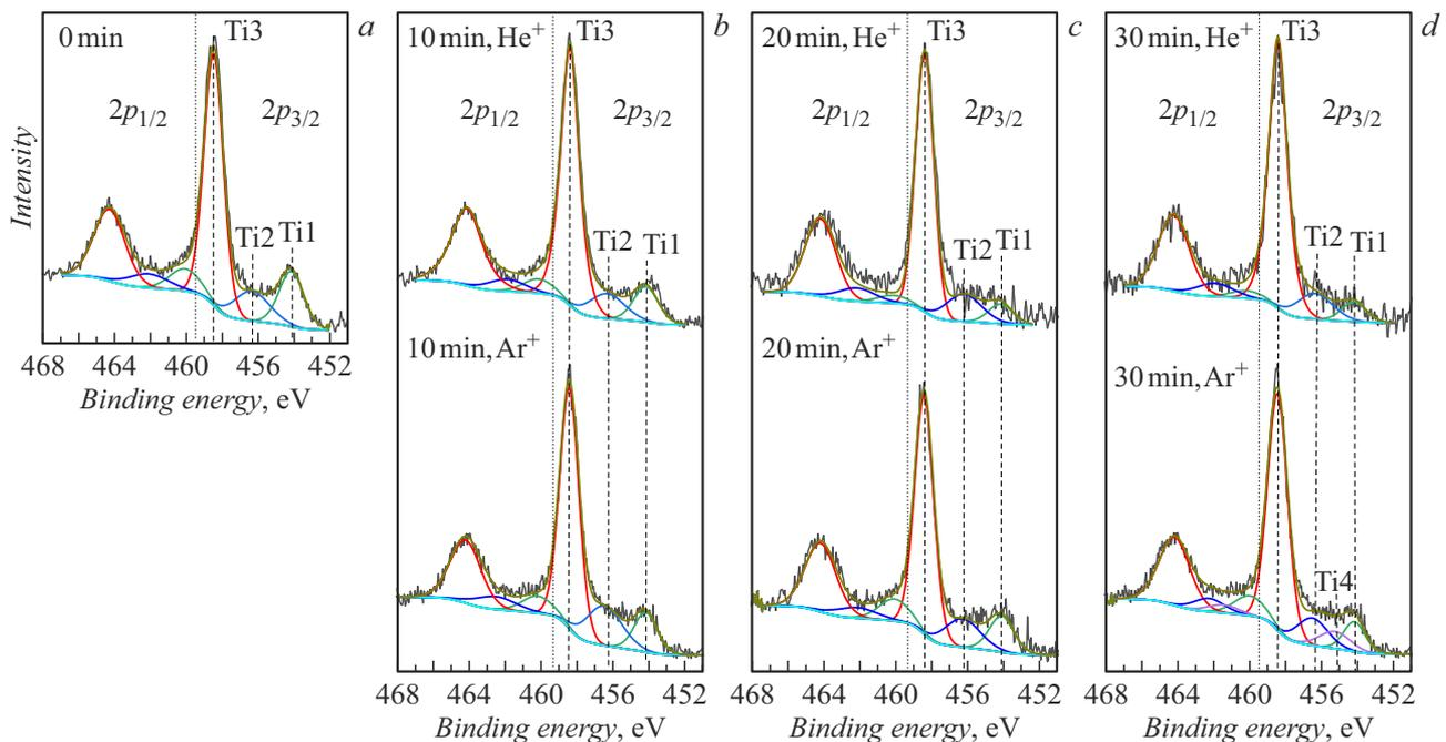
**Figure 5.** Ti  $2p_{1/2,3/2}$  PE spectra of the surface layer of „MWCNT/Ti“ samples: before irradiation (a) and after 10 (b), 20 (c) and 30 min (d) irradiation with helium and argon ions.
