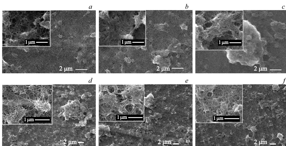
**Figure 2.** SEM images of the surface layer of „MWCNT/Ti“ system after 10 (a), 20 (b) and 30 min (c) irradiation with helium ions and after 10 (d), 20 (e) and 30 min (f) of irradiation with of argon ions.
