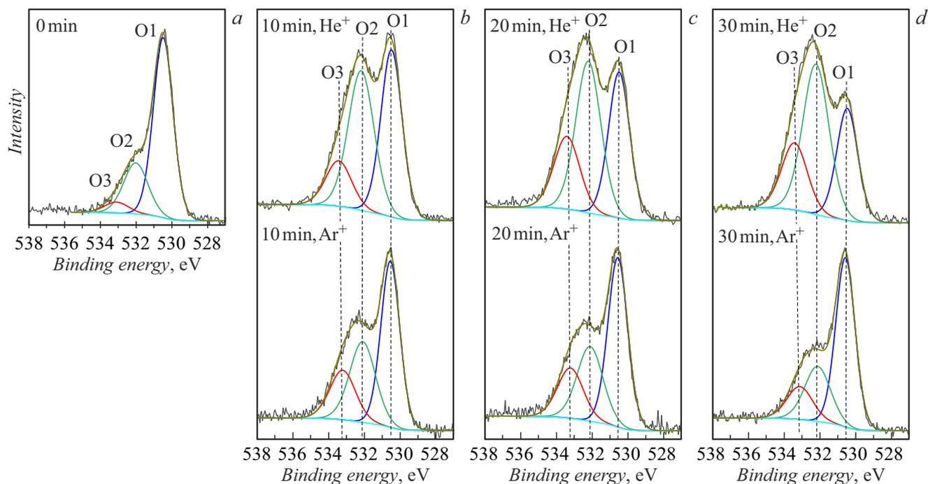
**Figure 6.** O 1s PE spectra of the surface layer of „MWCNT/Ti“ samples: before irradiation (a) and after 10 (b), 20 (c) and 30 min (d) irradiation with helium and argon ions.
