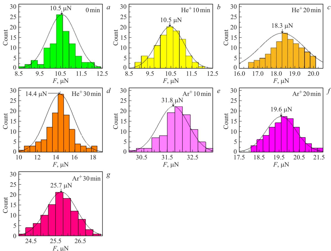
**Figure 3.** Histograms of the distribution of values of the adhesive strength of the MWCNT layer to the titanium substrate (a) before and after irradiation of the „MWCNT/Ti“ system with helium and argon ions for 10 (b,e), 20 (c,f) and 30 min (d,g).
