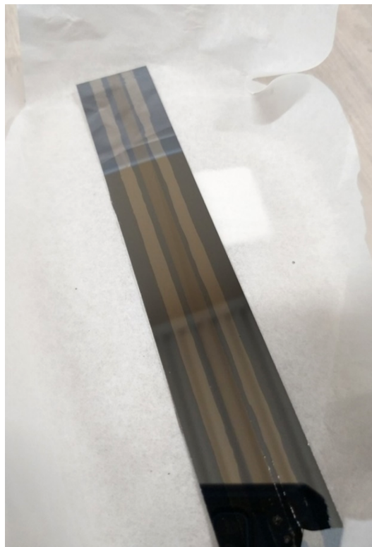
Figure 6. Experimentally obtained multi-strip multilayer mirror for the two-mirror monochromator of SKIF synchrotron.
