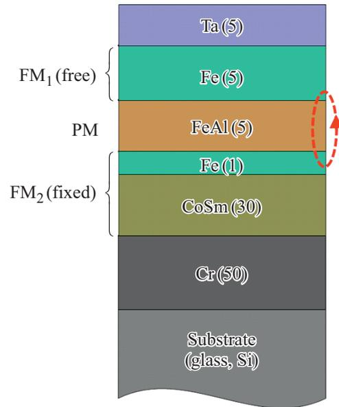
Figure 1. Scheme of the studied structure.
