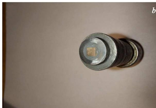
**Figure 1.** Internal structure of sensitive element of heterogeneous gradient heat flux sensor (*a*) and appearance of the sensor used in the insert (*b*).
