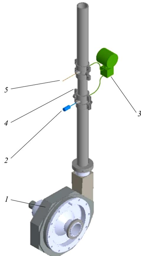
**Figure 1.** Diagram of the experimental bench: 1 — is the centrifugal charger; 2 — is the instrument KPDM-1 (Pitot-Prandtl tube connected to a micro pressure gage); 3 — ELEMER AIR-30 S3 CD-4 (differential pressure transducer); 4 — is the studied sample with porous element; 5 — is the thermocouple KTHA 02.01-062-K1-and-E310-1,5-100/2000.
