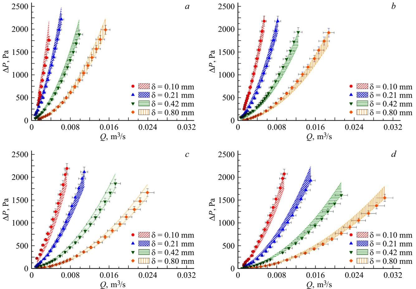
**Figure 3.** Experimental and calculation dependencies of the air pressure drops at MR on the flow rate for the samples differed by the wire diameter and porosity: *a* — porosity of 70%; *b* — 75%; *c* — 80%; *d* — 85%.
