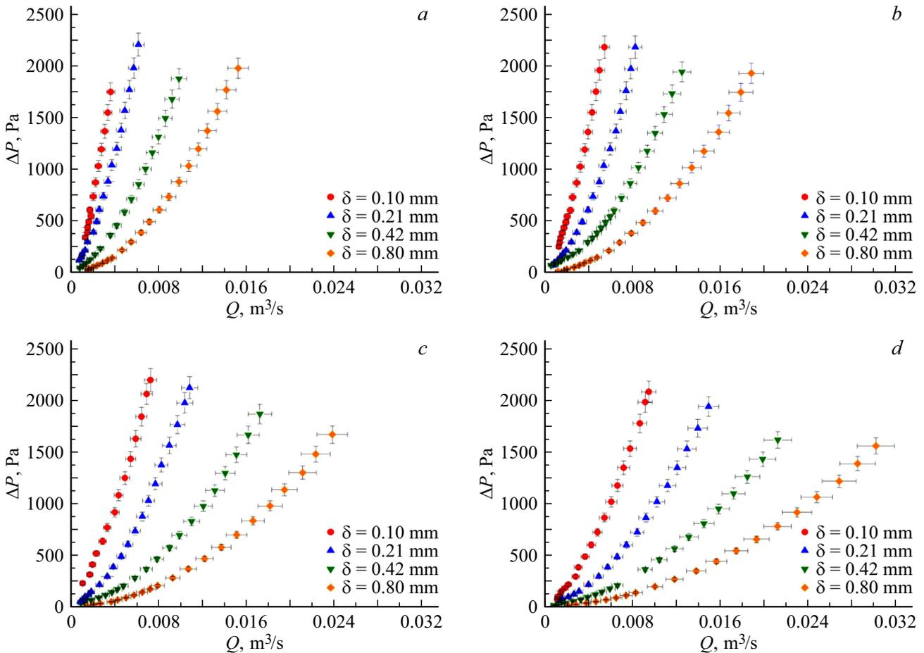
**Figure 2.** Experimental dependencies of the air pressure drop at MR on the flow rate for the samples differed by the wire diameter and the porosity: *a* — porosity of 70%; *b* — 75%; *c* — 80%; *d* — 85%.
