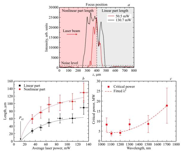
**Figure 3.** (*a*) Example of identifying "linear" and "nonlinear" plasma channel length for 1300 nm and a mean power of 50.5 mW and 130.7 mW by the luminous intensity profiles of the channel on the z axis; (*b*) "linear" and "nonlinear" plasma channel lengths for 1300 nm pumping; (*c*) dependence of the critical self-focusing power  $P_{\rm cr}$  on the pumping wavelength (red dots) and its approximation by function quadratic in wavelength (red dashed line).
