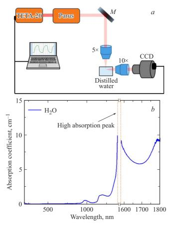
**Figure 1.** Experimental setup (a) and mid-IR absorption spectrum of water (b). Breakage at 1400–1580 nm is caused by the strong absorption band of water.
