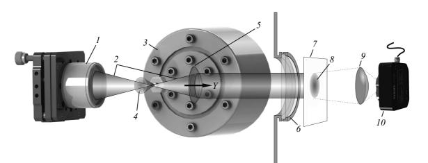
**Figure 1.** Scheme of the experimental setup. (1) — focusing lens, (2) — Nd:YAG laser beam, (3) — gas-jet target generator, (4) — supersonic Xe microjet, (5) — the lens converting the diverging laser beam into the parallel one, (6) — the glass window of the vacuum chamber, (7) — scattering screen, (8) — the image of the beam cross section on the screen, (9) — the lens to transfer the image to a CCD matrix, and (10) — the CCD sensor.
