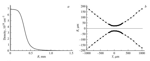
**Figure 2.** (*a*) The radial distribution of the concentration of Xe atoms in the target jet at the distance of 1mm from the nozzle exit and at the pressure  $P_0 = 13$  atm before the nozzle entrance. The point R = 0 is located on the jet axis. (*b*) Effective radius of the laser beam as a function of coordinate *Y* (along the beam axis). Black dots represent the effective beam radii measured using the photosensitive CCD matrix.
