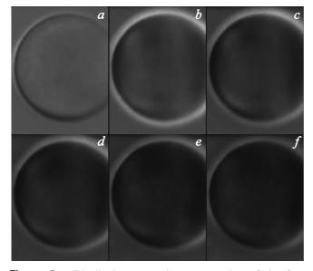
**Figure 5.** Distributions over the cross section of the fraction of absorbed laser energy,  $W_{abs}/W_0$ , for (a) - Y = 0,  $(b) - Y = 200 \,\mu$ m,  $(c) - Y = 400 \,\mu$ m,  $(d) - Y = 600 \,\mu$ m,  $(e) - Y = 800 \,\mu$ m,  $(f) - Y = 1000 \,\mu$ m.
