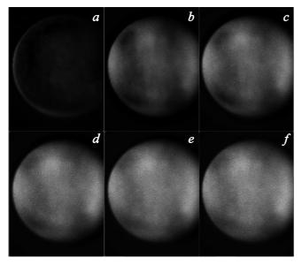
**Figure 4.** Distribution of the absorbed energy density,  $W_{abs} = W_0 - W_{tr}$ , over the laser beam cross section for: (a) — Y = 0, (b) —  $Y = 200 \,\mu$ m, (c) —  $Y = 400 \,\mu$ m, (d) —  $Y = 600 \,\mu$ m, (e) —  $Y = 800 \,\mu$ m, (f) —  $Y = 1000 \,\mu$ m.
