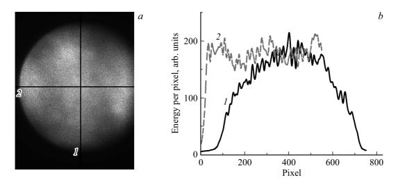
**Figure 3.** (*a*) Energy distribution over the cross section of the IR laser beam as recorded with the CCD sensor; (*b*) distributions along two mutually perpendicular diameters: the vertical diameter (I) and the horizontal one (2).
