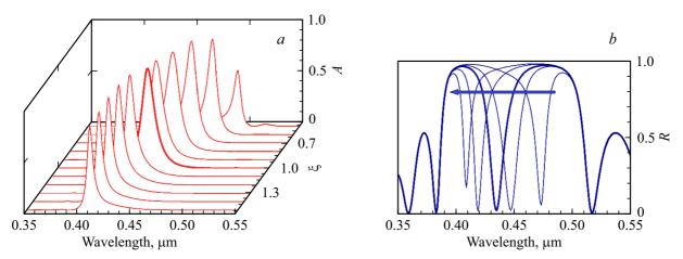
**Figure 3.** Dependence of the absorption spectra (a) and reflection spectra (b) of the photonic structure on the aspect ratio  $\xi$  in silver NPs. In the figure (b), the aspect ratio of NPs takes values of 0.6, 0.8, 1, 1.2, 1.5, the direction of increase  $\xi$  is shown by an arrow. Interparticle distance p = 130 nm.
