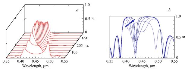
**Figure 2.** Dependence of the absorption spectra (a) and reflection spectra (b) of the photonic structure on the interparticle distance p in a two-dimensional array of silver NP. In the figure (b), the interparticle distance takes values of 30, 55, 105, 180, 280, 380 nm, the direction of increase p is shown by an arrow. Aspect ratio of NP  $\xi = 1$ .
