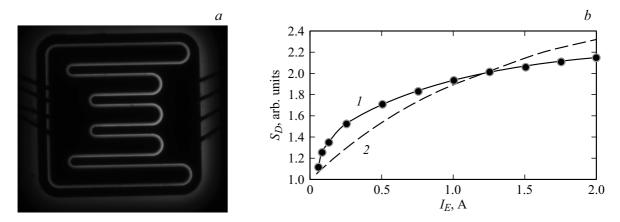
**Figure 2.** (a) RL intensity profile of the KT504A transistor at a current of 1.5 A in diode mode, (b) dependence of the coefficient of heterogeneity of the RL intensity distribution along the emitter track on the emitter current: 1 — measurement result, 2 — calculation result.
