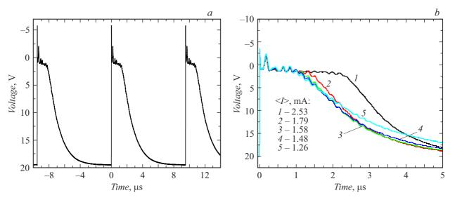
**Figure 3.** a — The time dependence of capacitor voltage in the maximum repetition rate mode. b — time dependence of the capacitor voltage for different average power supply currents  $\langle I \rangle$ . Blocking voltage is 20 V, thyristor key based on HeT structure, capacitor capacitance is 1 nF.
