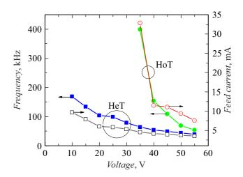
**Figure 1.** Dependences of the maximum frequency of generation of current pulses in the thyristor-capacitor circuit, as well as the average supply current on the blocking voltage for thyristors based on HoT and HeT structures. The capacitance of the capacitor is 1 nF.
