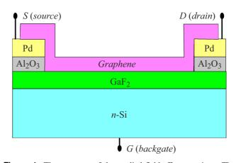
**Figure 1.** The structure of the studied field-effect transistor. The graphene film serves as a current-conducting layer, and fluoride — as a gate insulator (earlier, other combinations of materials were used in such devices:  $MoS_2/hBN/Si$ , etc.).
