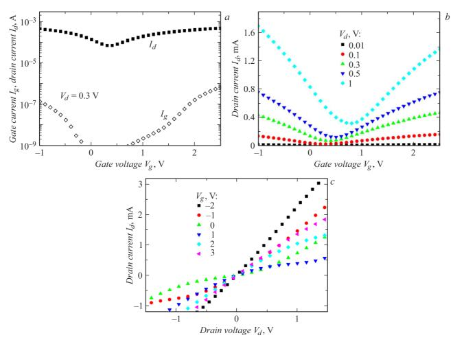
**Figure 2.** Typical characteristics of transistors with graphene over CaF<sub>2</sub>. a — comparison of the drain current and the leakage current through insulator; b — dependencies of the drain current on the voltage at the gate for several given drain voltages; c — dependencies of the drain current on the drain—source voltage for several given voltages of the gate. For all parts of Figure, the size of the channel is  $L \times W = 80 \times 50 \,\mu$ m, the temperature is 25°C.
