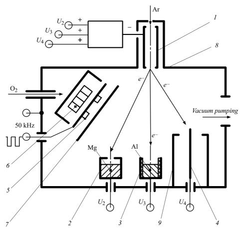
**Figure 1.** Schematic diagram of thin film deposition setup MgAl<sub>2</sub>O<sub>4</sub>: self-pumped cathode (1), crucibles (2, 3), rod-type anode (4), samples (5), heater (6), shutter (7), vacuum chamber (8), screen (9).
