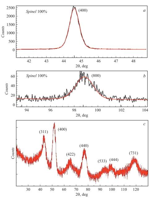
**Figure 2.** X-ray diffraction patterns of MAS film on Si substrate obtained in  $\theta - 2\theta$  line-scan mode (400) (*a*) and (800) (*b*) and in 5° sliding beam incidence mode (*c*).
