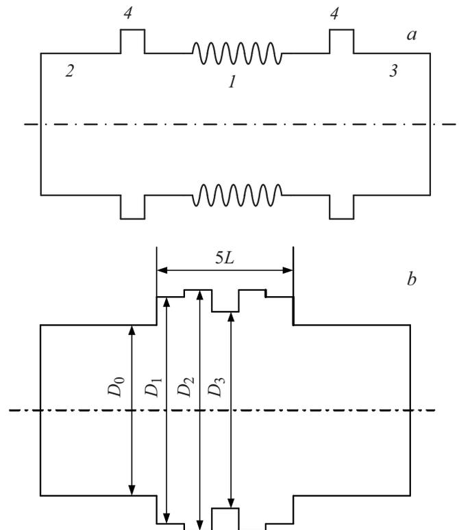
**Figure 1.** Schematic diagram of the electrodynamic system of a powerful microwave generator of ultrashort pulses. *a* — general scheme: 1 — interaction space, 2 — electron beam input, 3 — waveguide for radiation output, 4 — selective reflectors. *b* — simulated profile of a selective broadband five-stage reflector 4.
