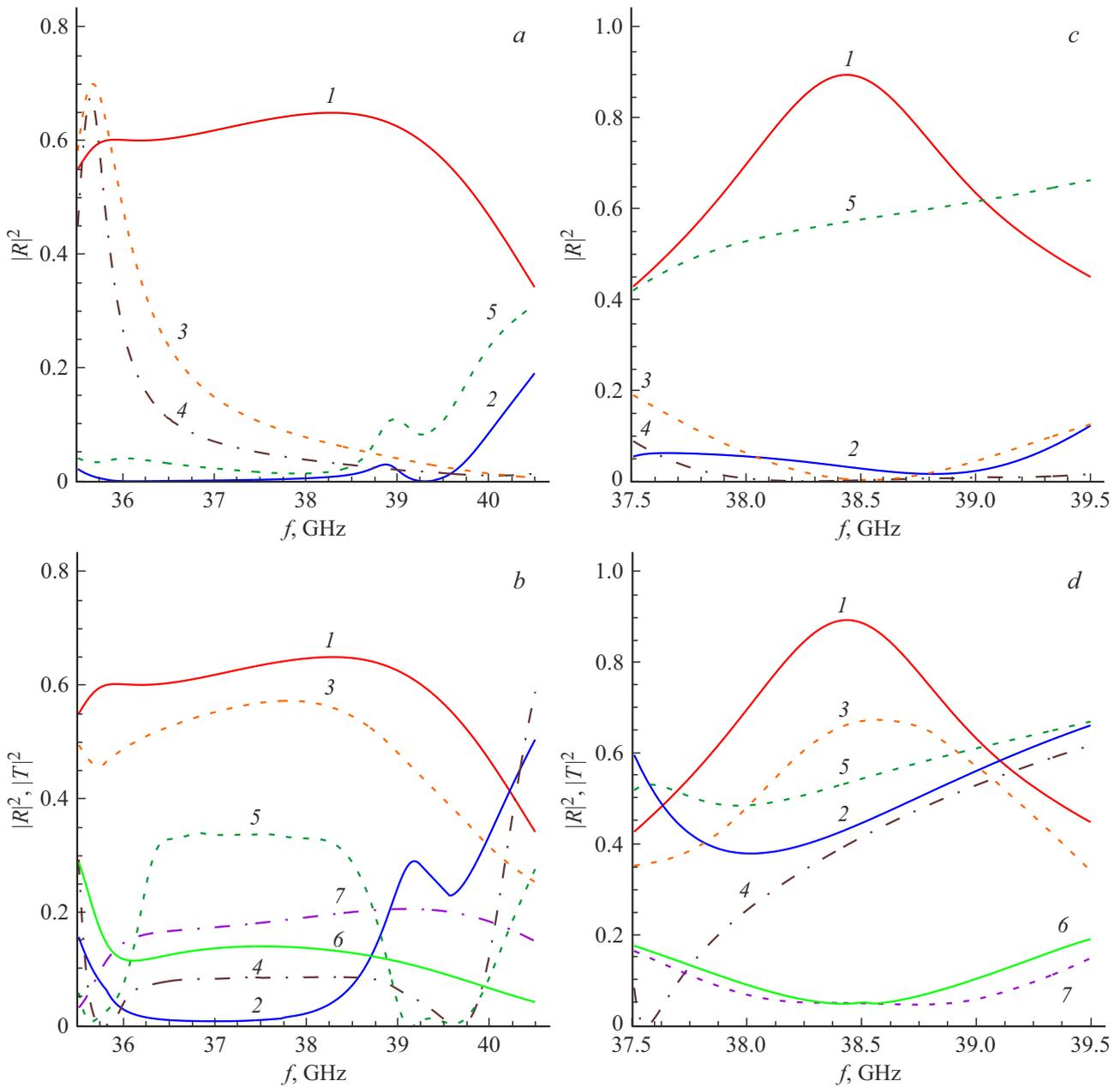
**Figure 2.** Frequency dependencies of reflectors with the maximum reflection levels 0.65 (*a,b*) and 0.9 (*c,d*). *a,c* — mode reflection  $E_{02}$  (1) and the lowest modes  $H_{11}$  (2),  $E_{01}$  (3),  $H_{21}$  (4),  $E_{11}$  (5); *b,d* — mode reflection  $E_{02}$  (1), reflection of higher modes  $H_{31}$  (2),  $E_{21}$  (3),  $H_{12}$  (4),  $E_{12}$  (5) and mode transformation  $E_{02}$  to the mode  $E_{01}$  reflected (6) and transmitted (7).
